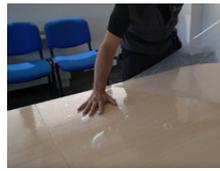
6. Turn the film over and apply the adhesive surface to the substrate (2 people if large surface). Adjust the position of the film by sliding it.
