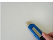
1. Lift the corner with a cutter, taking care not to damage the support.
