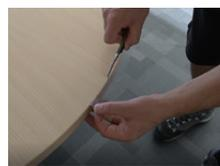
9. If necessary (complex shape), cut off the excess film with a cutter (3mm back from the edge of the substrate). Do not apply too much pressure as this may scratch the holder.
