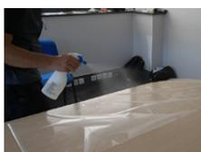
5. Thoroughly moisten the adhesive surface with soapy water using a spray or atomizer.
