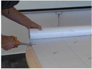
1. Cut the film to the required size considering overflows.
